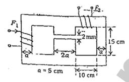
Core thickness = 8 cm  $\mu$  for iron = 2500  $\mu_0 = 4\pi \times 10^{-7}$
